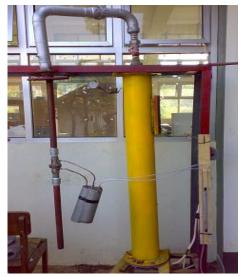
Gambar 2. Alat pengukuran primary flow
